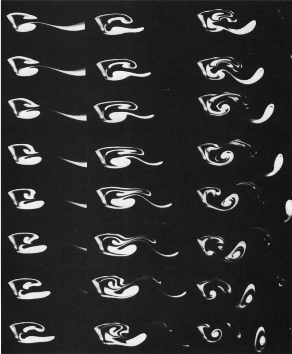
FIGURE 3. \alpha = 60^\circ , R = 124 , t_1^* = 11 , \Delta t^* = 0.214 , c = 1.27 cm, 64 frames/s, airfoil in reverse.
