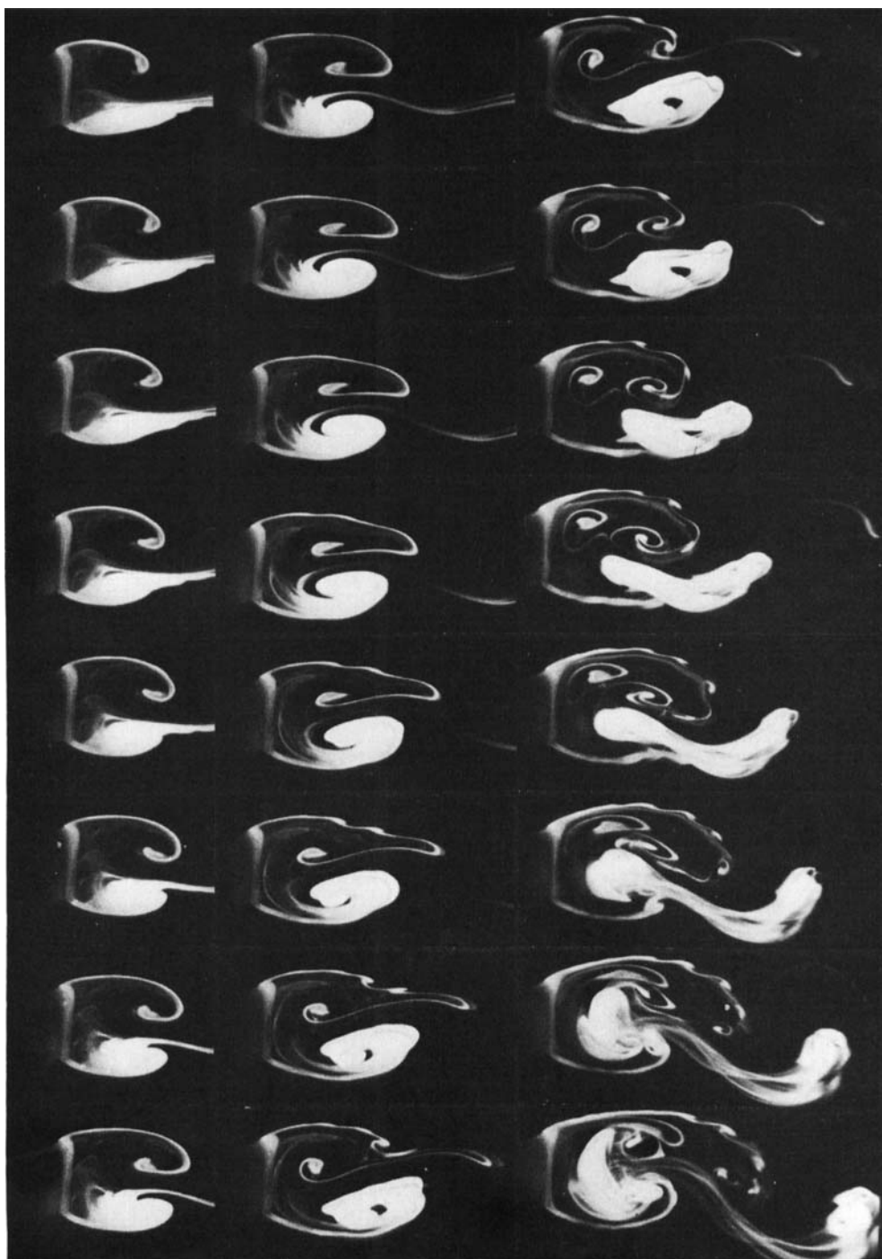
FIGURE 1. Accelerated flow around an airfoil. \alpha = 90^\circ , R = 350 , t_1^* = 5.6 , \Delta t^* = 0.15 , c = 2.54 cm, 64 frames/s.
